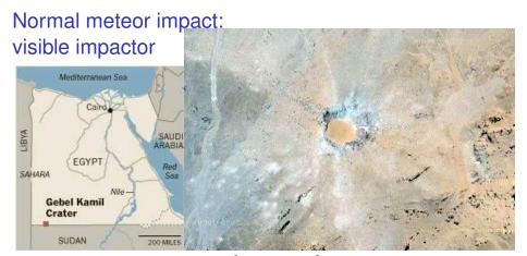
Iron-nickel (20%) Gebel-Kamil: 22<sup>0</sup>01'06"N, 26<sup>0</sup>05'16"E East Uweinat Desert, Egypt: 44.8m in diameter, 15.8m deep meteorite crater: 1600 kg of iron meteorite shrapnel, 3400 kg >10 g pieces remained today. Upon hypervelocity impact, the 1.3 meters wide 5 to 10 tons meteorite was disrupted into thousands of fragments located up to 200 m from the crater rim, largest known fragment 83 kg. Dated to about 4,500 years, explored first 2009/10. A possible source of Egypt-Pharaoh Iron.
